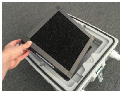
Fig. 4: Changing the active carbon filter
